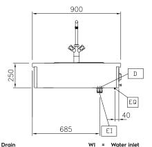
D Drain DO Overflow drain pipe ΕI Electrical inlet (power)
